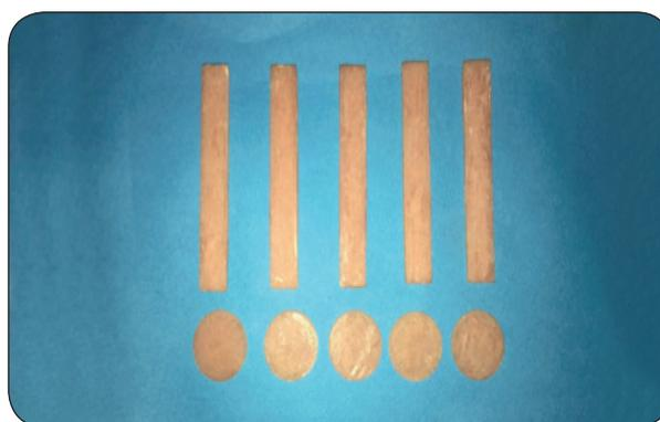
Fig. (3) Finished specimens of PMMA modified by 5% Henna.
