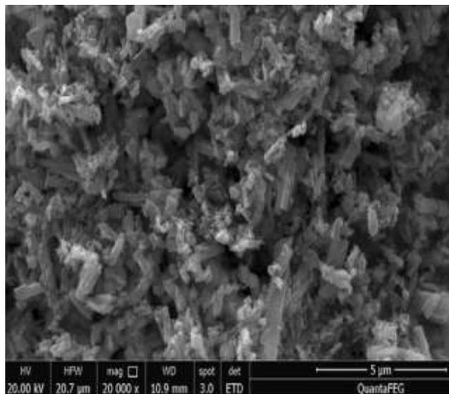
Figure 2: SEM of prepared ZnO nanoparticle
