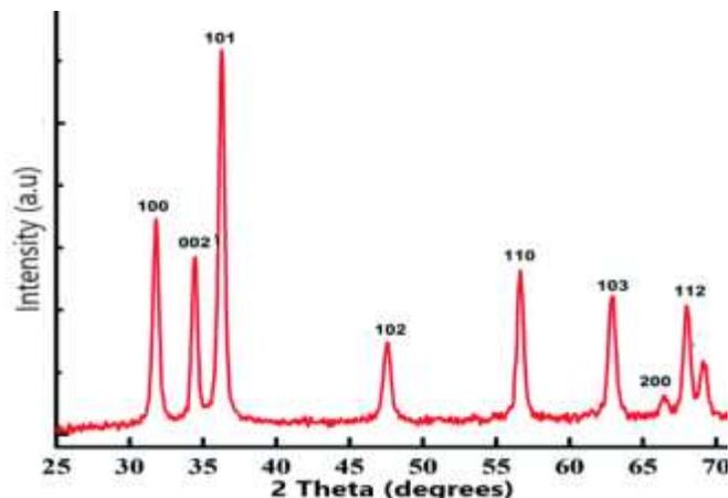
Figure 1: XRD pattern for ZnO nanoparticle
