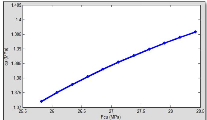
**Figure 25: Relation between (fcu) and Shear Strength**
