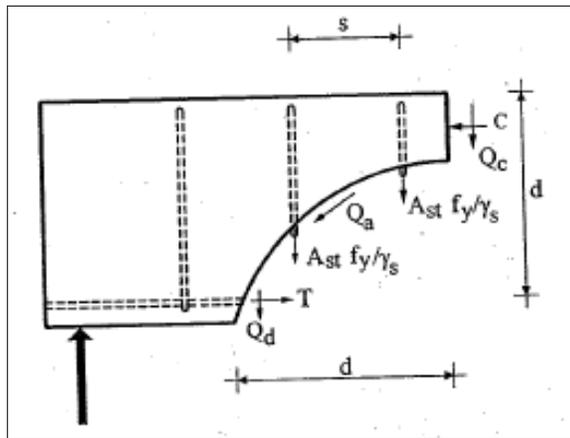
**Figure 1: Forces at Diagonal Crack of Reinforced Concrete Beam**
