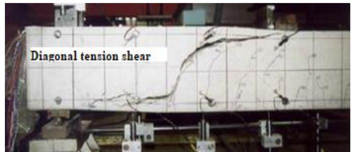
**Figure 2: Shear Failure in a Beam Reinforced with FRP without Transverse Reinforcement**
