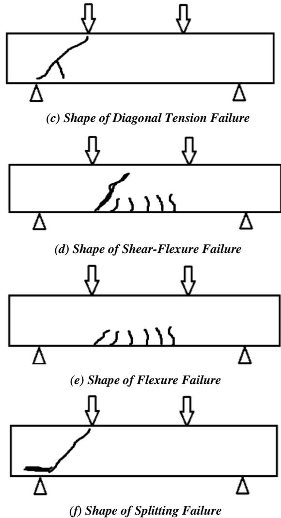
**Figure 4: Modes of failure**
