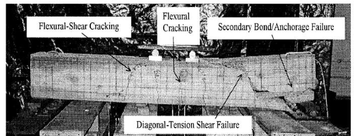
**Figure 3: Typical FRP Shear Failures**
