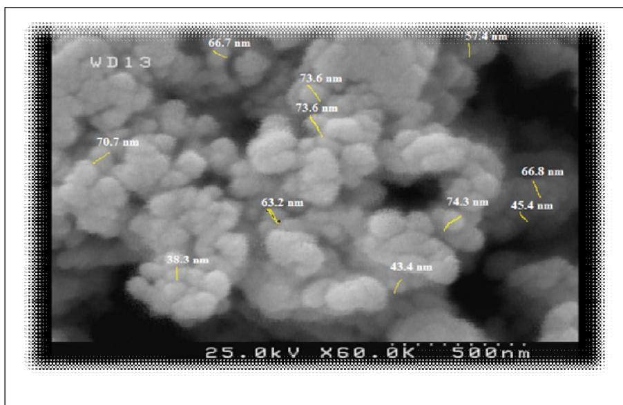
Figure: 8 SEM image of silver nanoparticles prepared with *Carissa* extract
