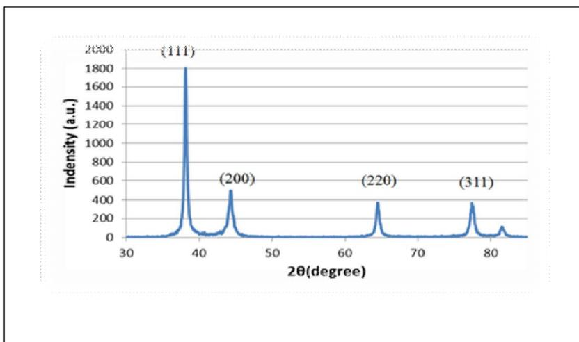
Figure:7 X-ray diffraction pattern of silver nanoparticles Prepared with *Carissa* extract
