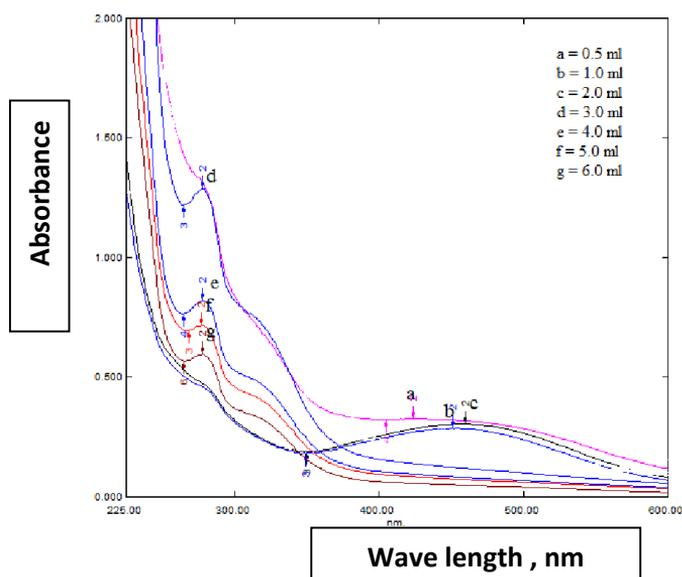
Figure:1 UV-vis spectra of silver nanoparticles at different concentration of *Carissa* extract
