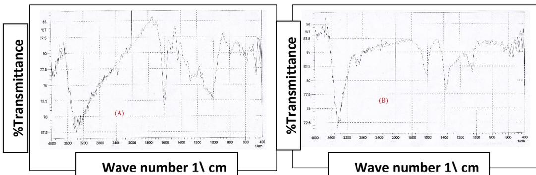
Figure: 6 FTIR spectra of capped silver nanoparticles
