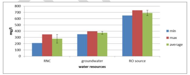
**Figure 1.**Total dissolved solids of different water resources used for drinking water production through studying period of March, 2017 and June, 2018.
