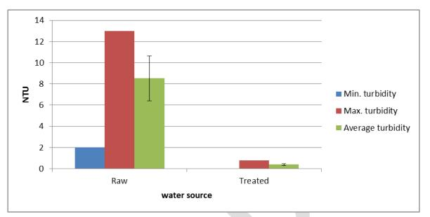
**Figure 2.**Turbidity of different water source of Badr station for drinking water production through studying period of March, 2017 and June, 2018.
