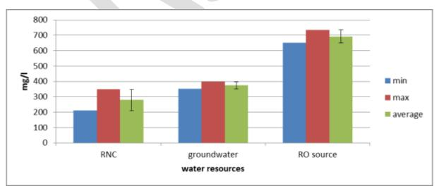
Figure 1: Total dissolved solids of different water resources used for drinking water production through studying period of March, 2017 and June, 2018.
