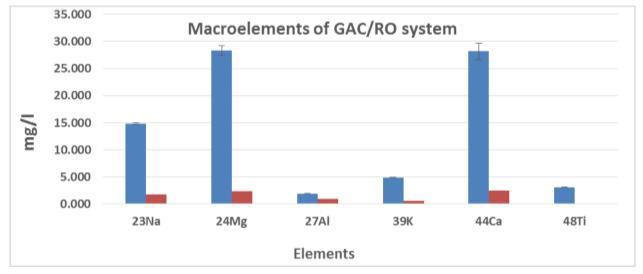
**Figure 4:** Macroelements composition of water before and after application of GAC/RO system ofBerkash region, Giza, Egypt stations for drinking water production through studying period of March, 2017 and June, 2018.
