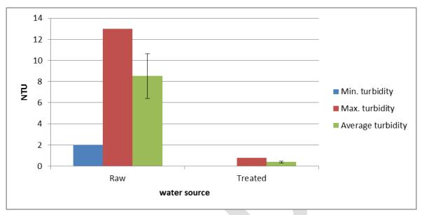
Figure 2: Turbidity of different water sourceof Badr station for drinking water production through studying period of March, 2017 and June, 2018.
