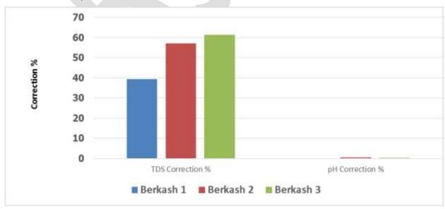
**Figure 3:** Water properties correction as a results of GAC/RO system ofBerkash region, Giza, Egypt stations for drinking water production through studying period of March, 2017 and June, 2018.
