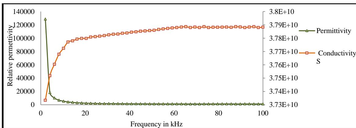
Figure (7): The variations of the relative permittivity ( $\epsilon'$ ) and electric conductivity ( $\sigma$ ) as a function of frequency in the range 0.1-100kHz for sample bacterial suspension exposed to 0.6 SMF for one hour.
