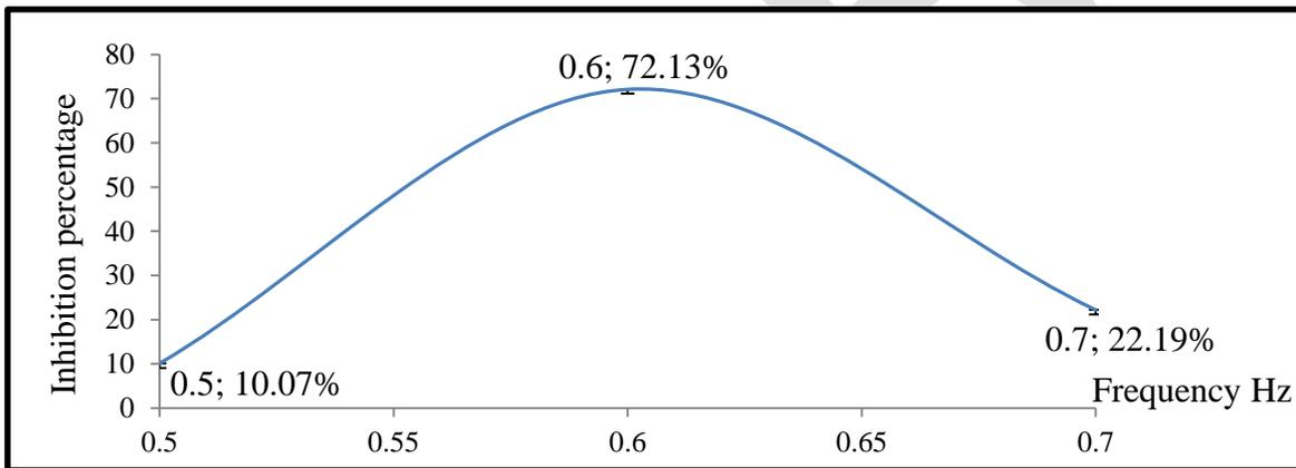
Figure (3): Inhibition percentage of the exposed samples with respect to control at different frequencies SMP and fixed time 30 minutes (at the 8<sup>th</sup> hour of incubation).
