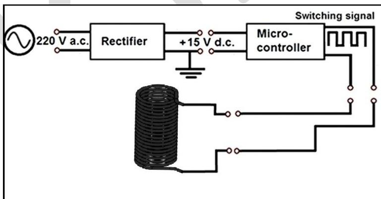
Figure (1): Schematic illustration of the experimental design used for exposure.
