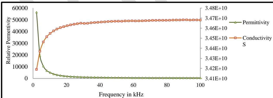
Figure (6): The variations of the relative permeability ( $\epsilon'$ ) and electric conductivity ( $\sigma$ ) as function of frequency in the range 0.1-100kHz for control sample bacterial suspension.
