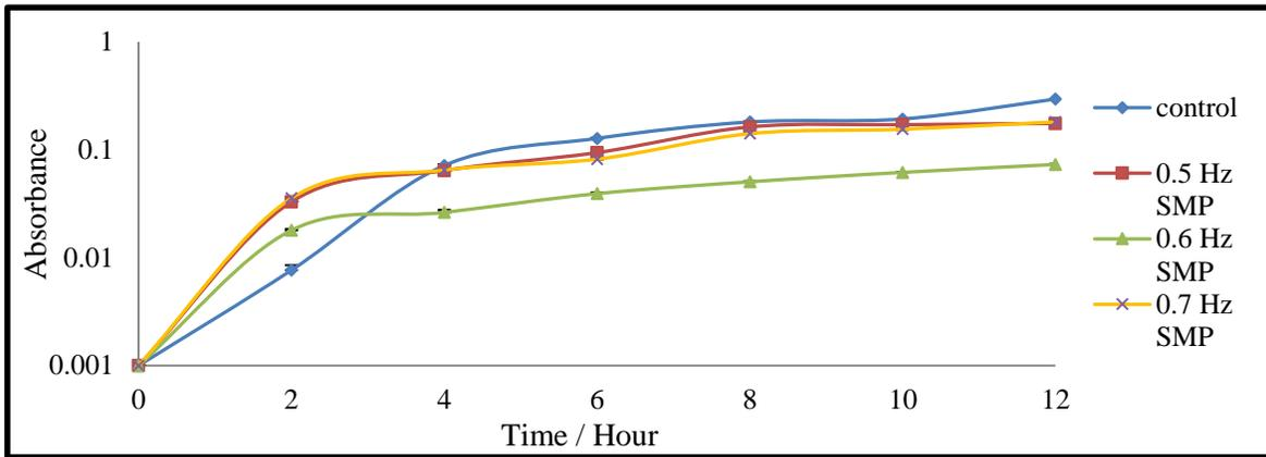
Figure (2): The growth curve of *P. mirabilis* exposed to different frequencies SMP for a period of 30 minutes.
