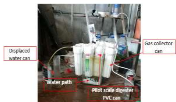
Fig. 1. Pilot scale batch PVC cans (anaerobic digester)
