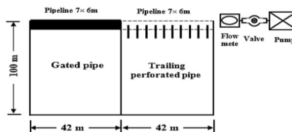
**Figure 1. The experiments Layout**
