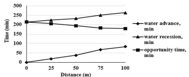
**Figure 4. Advance, recession and opportunity times curves for the trailing perforated pipe irrigation system.**
