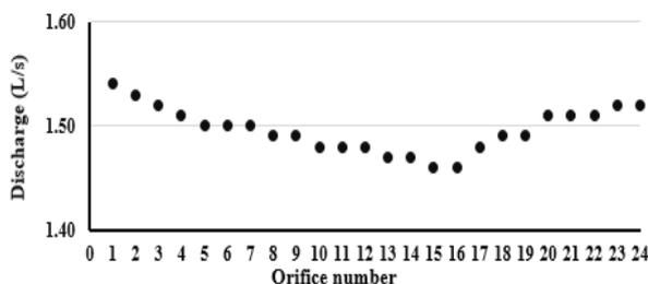
**Figure 2. Trailing perforated pipe irrigation system performance evaluation.**
