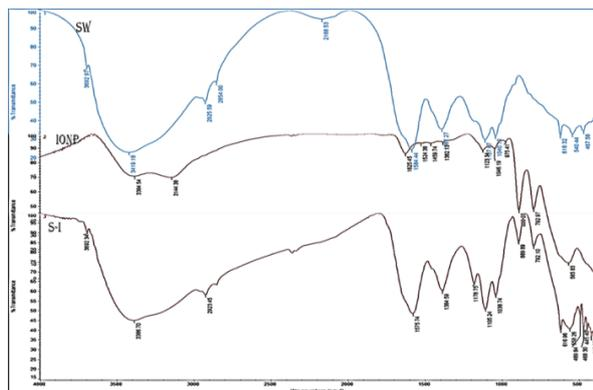
Figure 1. FT-IR spectrums for Seaweed (SW), Iron oxide nanoparticles (IONP) and seaweed-iron oxide nanoparticles composite (S-I)
