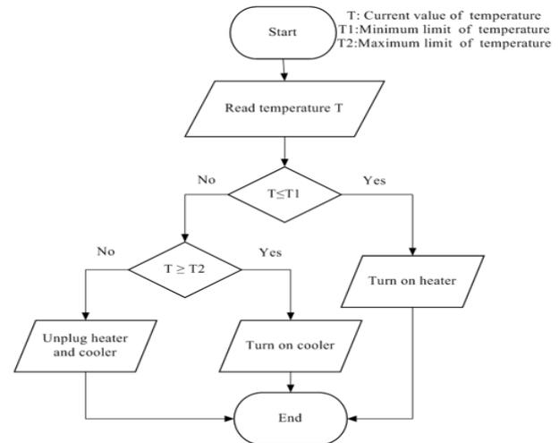
**Fig. 4. Flow chart for the temperature control subroutine.**
