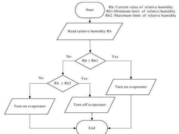
**Fig. 5. Flow chart for the relative humidity control subroutine.**
