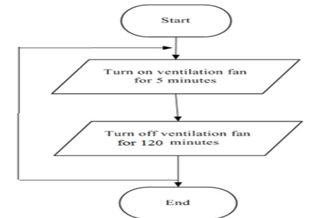
**Fig. 6. Flow chart for the ventilation control subroutine.**
