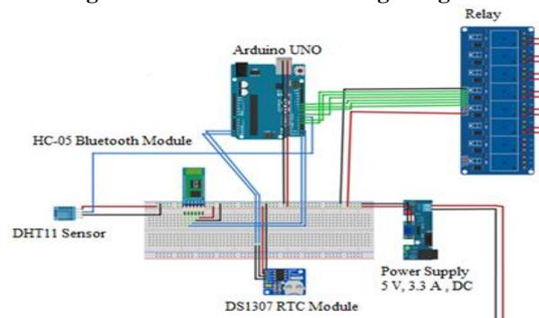
**Fig. 3. Diagram showing how to connect the Arduino board to the electronic components.**
