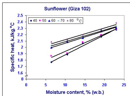
**Fig. (2):** Effect of moisture content on specific heat of sunflower seeds at different temperature levels.
