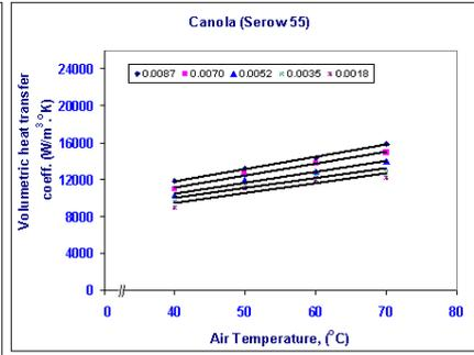
Fig (10): Effect of air temperature on heat transfer coefficient of canola seeds at different levels of mass air flow rate.
