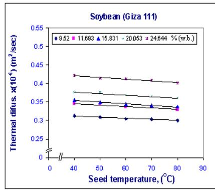
Fig (7): effect of seeds temperature on thermal diffusivity of soybean seeds at different levels of moisture content
