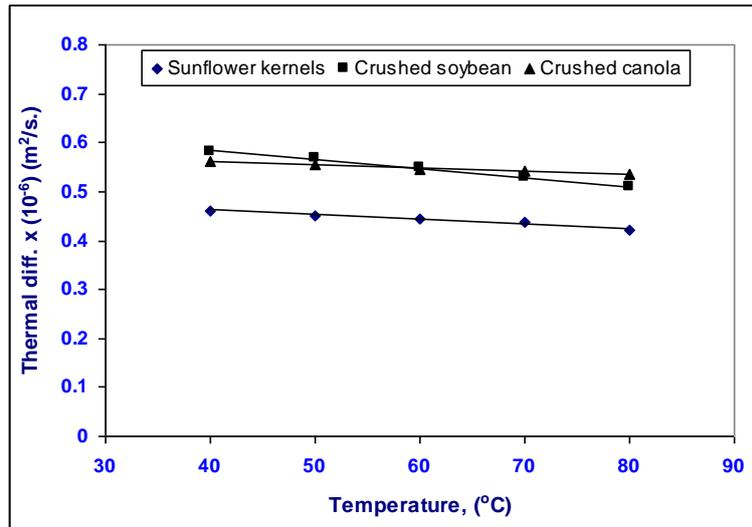
Fig (8): Effect of seeds temperature on thermal diffusivity of the crushed canola seeds.
