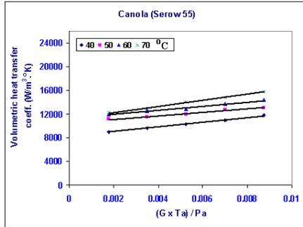
Fig (9): Effect of mass air flow rate on heat transfer coefficient of canola seeds at different levels of air temperature
