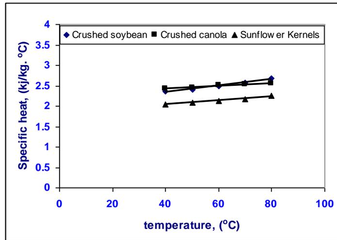
Fig (4): Effect of seeds temperature on specific heat for sunflowerkernels, crushed soybean and crushed canola.
