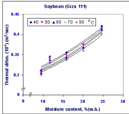
Fig (6): Effect of moisture content on thermal diffusivity of soybean seeds at different levels of temperature
