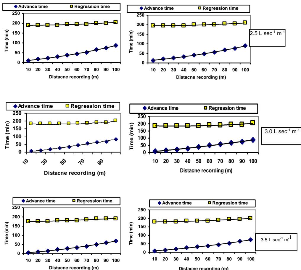
**Fig. (3):** The effect of width border and irrigation discharge on advance, recession, and opportunity time in the two seasons.
