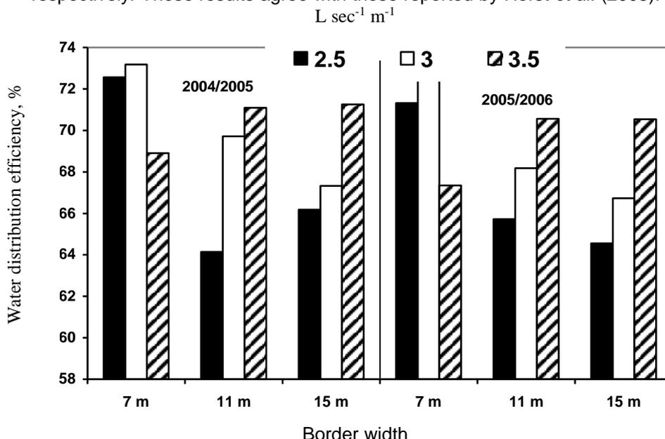
**Fig. (2): Values of water distribution efficiency (WDE%) under different treatments for wheat crop during growing seasons 2004/2005 and 2005/2006.**
