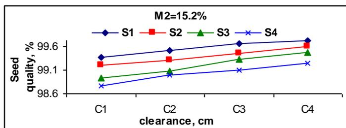
**Fig (3-2) Effect of disc-housing clearance on seed quality**
