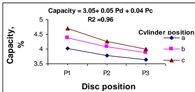
Fig (2-C) Effect of spikes position on disc and cylinder on separating Capacity .
