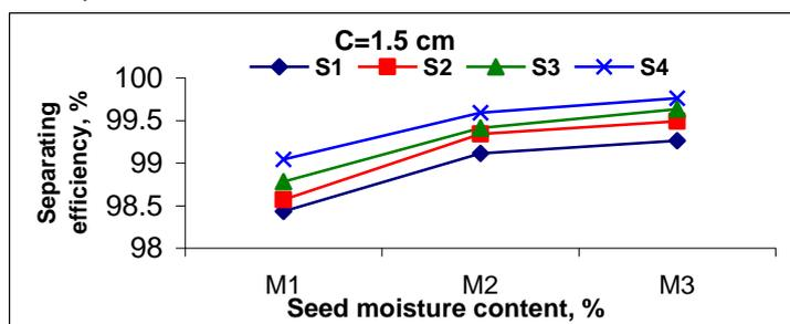
Fig (4-3) Effect of seed moisture content on separating efficiency
