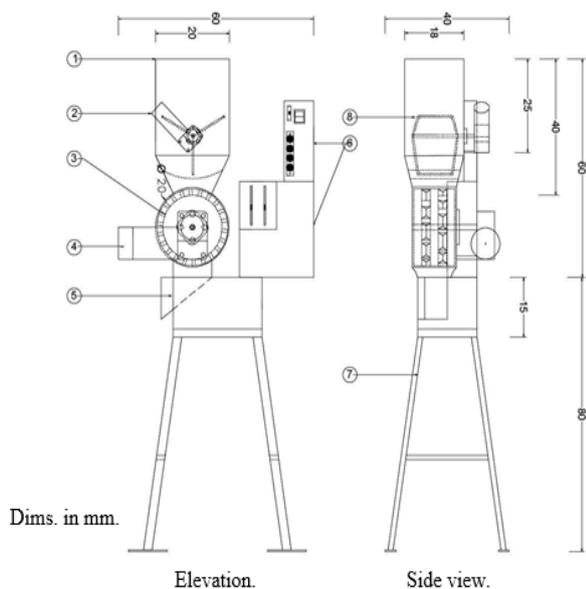
**Fig. 1. The test rig**
