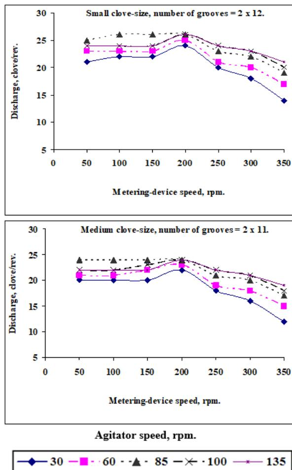
**Fig. 7. Effect of metering-device and agitator speeds on garlic-cloves discharge for small and medium clove-sizes.**
