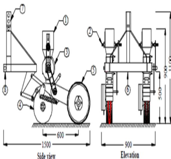
Fig. 6. Elevation and side views of the two-units garlic cloves planter.
