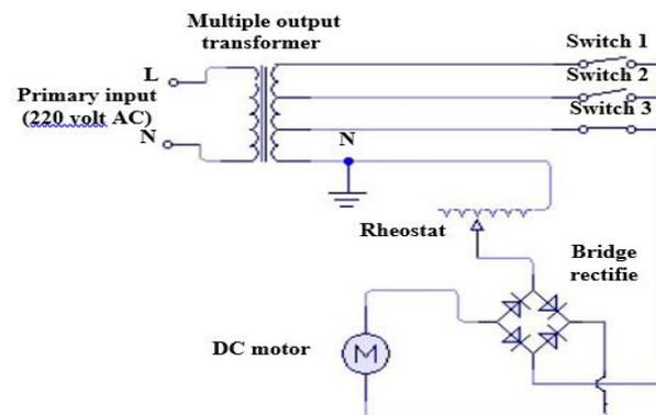
**Fig. 4. Power circuit of metering device.**
