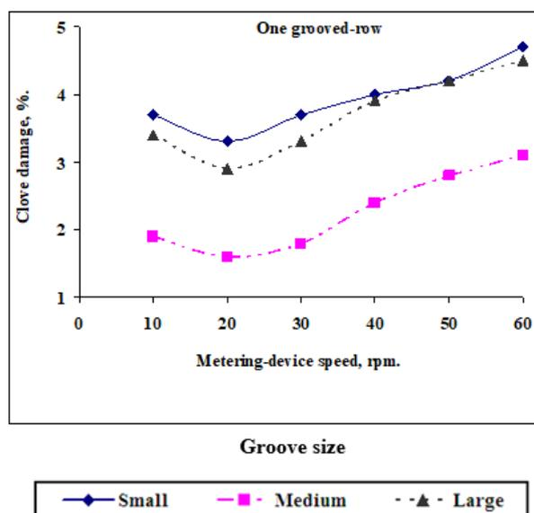
**Fig. 12. Effect of metering-device and groove size on garlic-cloves damage percent for one grooved-row metering device.**
