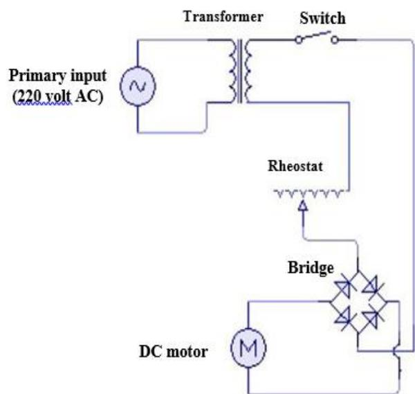
Fig. 5. Power circuit of agitator.
