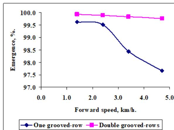
**Fig. 13. Effect of metering-device on plant-emergence percent for one grooved-row metering device.**
