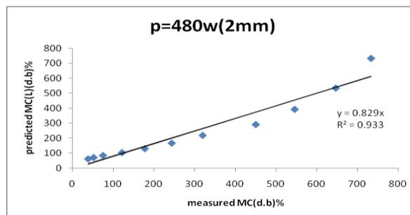
Figure 8. Measured and predicted values using Lewis model at thickness (2mm) and power (480w)
