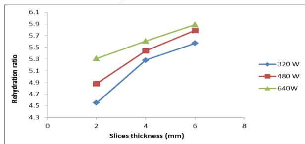
**Figure 10. Effect of different slices thickness on the rehydration ratio by microwave oven.**
