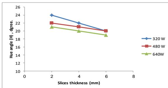
**Figure 9. Effect of different slices thickness on the hue angle at levels of microwave power by microwave oven.**
