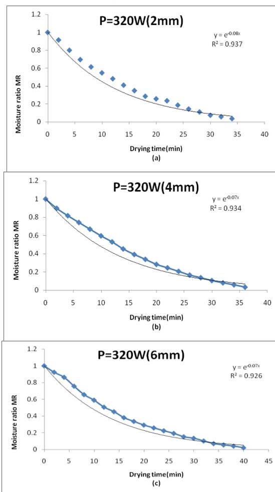
**Figure (2 a, b and c): The relationship between time (min) and MR to determination the (KL) constant of Lewis equation at the maximum power of 320 W and different slices thickness.**
