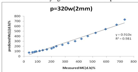
Figure 7. Measured and predicted values Lewis model at thickness (2mm) and power (320w)
