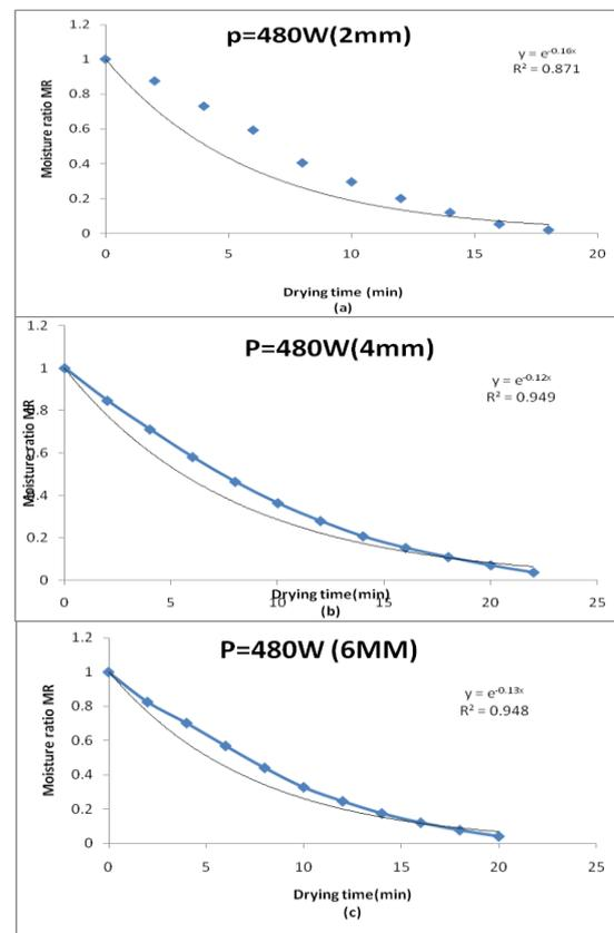
**Figure (3 a, b and c): The relationship between time (min) and MR to determination the (KL) constant of Lewis equation at the maximum power of 480 W and different slices thickness**
