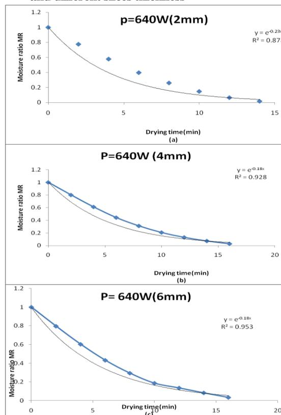
**Figure (4 a, b and c): The relationship between time (min) and MR to determination the (KL) constant of Lewis equation at the maximum power of 640W and different thickness of slices**
