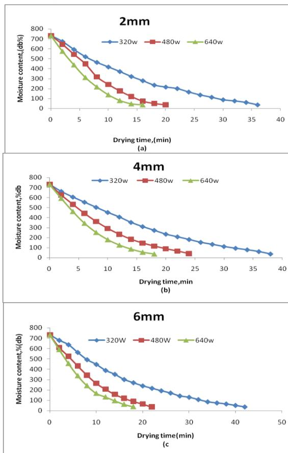
Figure (1 a, b and c) The moisture constant of onion via drying time at slices thickness and microwave power.
