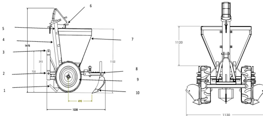
**Fig. 1. Schematic diagram of main components for a single-row automatic potato planter**
