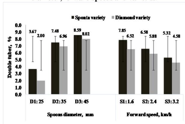
**Fig. 4. The double tubers ratio as affected by spoons diameter, forward speeds and varieties.**
