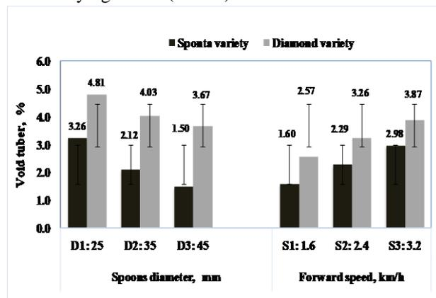
**Fig. 3. The void tuber ratio as affected by spoons diameter, forward speeds and varieties.**
