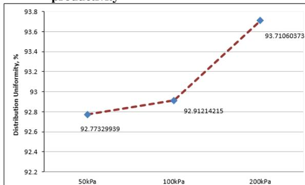
**Fig. 6. The relationship between pressure and distribution uniformity**
