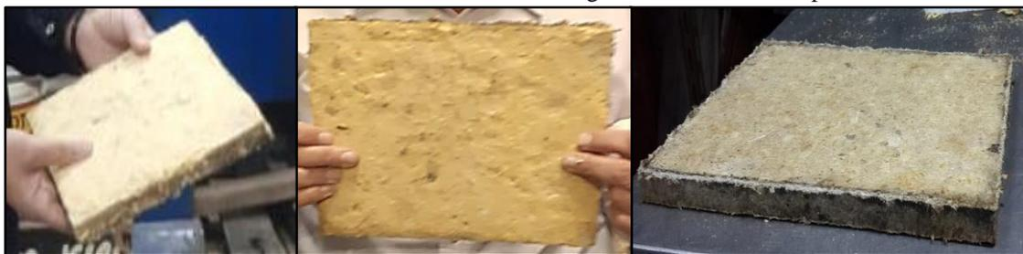
**Fig. 4. Manufactured particle boards**
