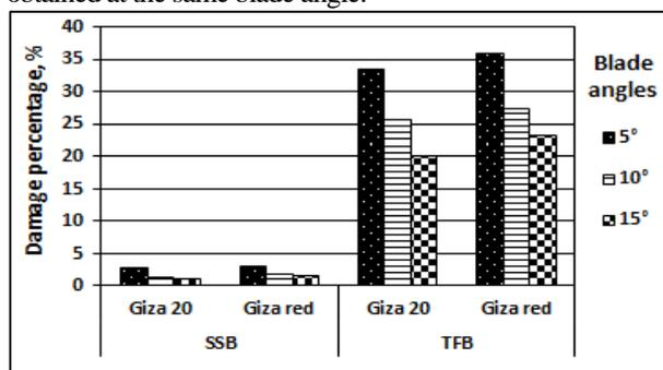
**Fig. 5. Effect of blade type and blade angle on the damaged bulbs percentage for the two onion cultivars**
