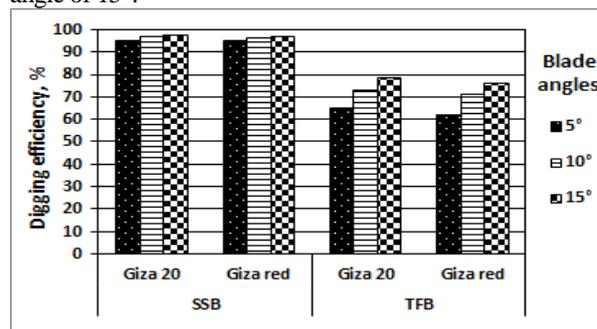
**Fig. 6. Effect of blade type and blade angle on digging efficiency during digging the two onion cultivars**
