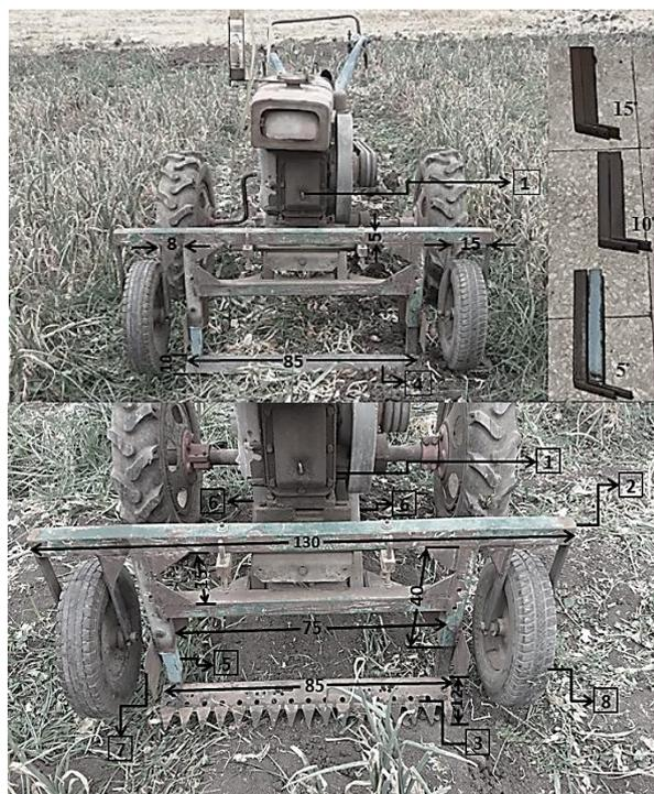
**Fig. 1. A view of the developed onion digger with the two-wheel tractor**
