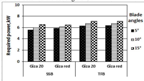
Fig.7. Effect of blade type and blade angle on the required power for the two onion cultivars
