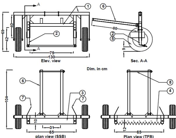
**Fig. 2. Schematic diagram of the developed onion digger**
