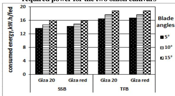
Fig. 8. Effect of blade type and blade angle on energy consumption for the two onion cultivars
