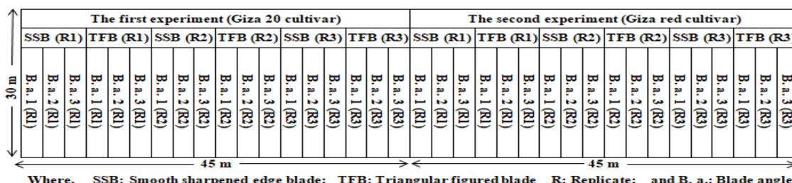
Where, SSB: Smooth sharpened edge blade; TFB: Triangular figured blade R: Replicate; and B. a.: Blade angle
