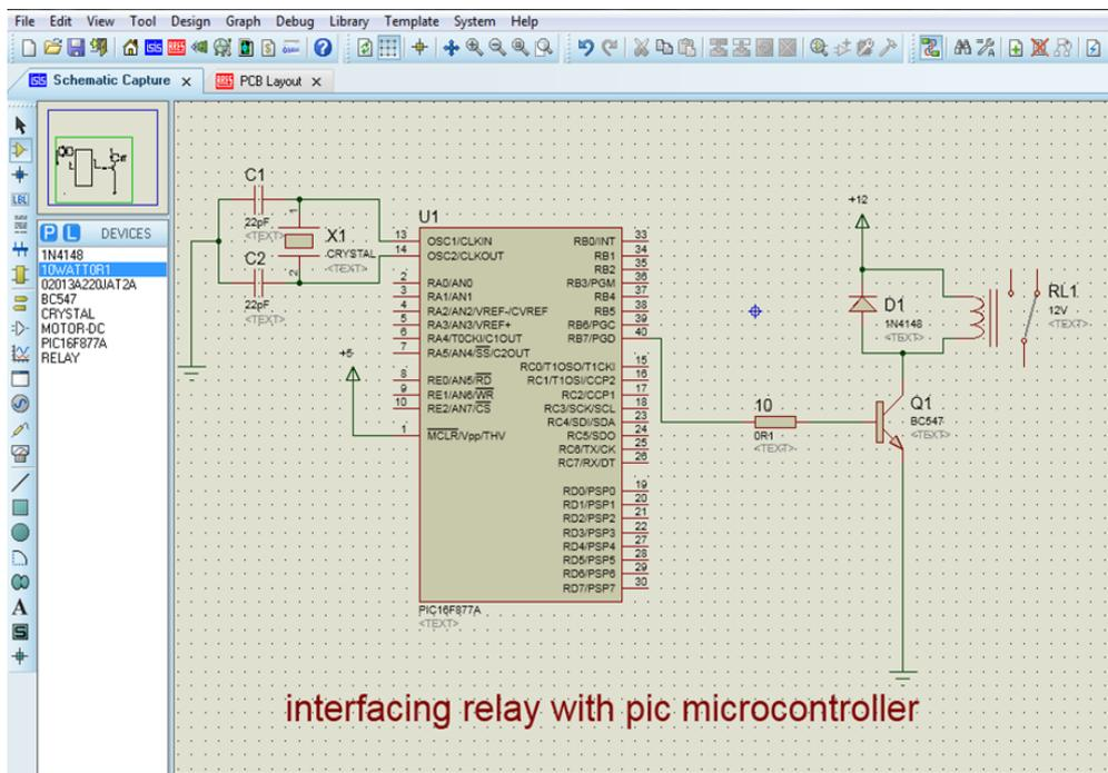
**Fig. 4. interfacing relay with pic microcontroller**
