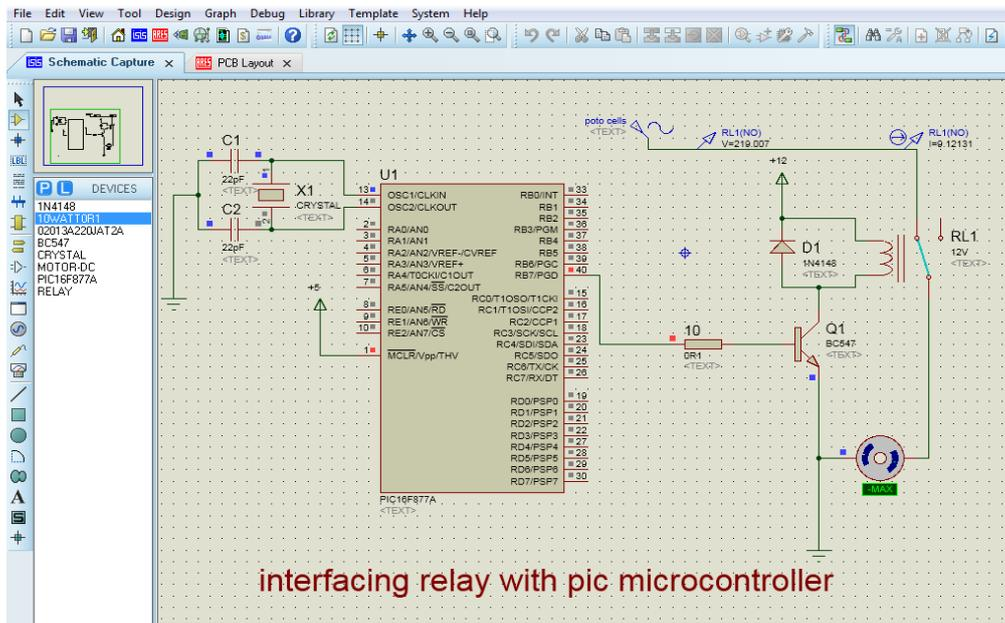
**Fig .1. Schematic diagram in Proteus**
