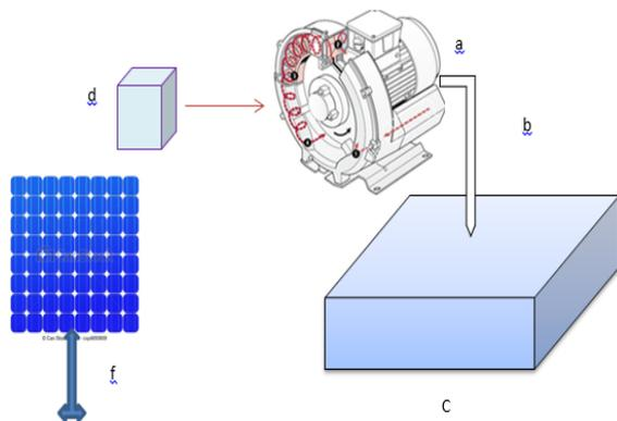
**Fig. 2. View of a pumping air system showing (a) AC motor + Air pump, (b) tube, (c) fish tank, (d) motor controller, (f) photovoltaic system.**
