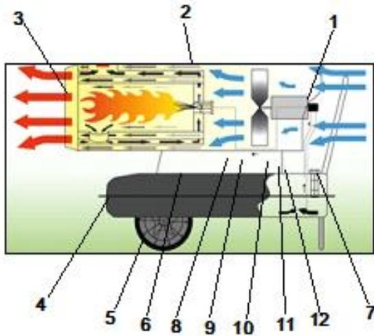
Fig .3. Heat paths in the burner
