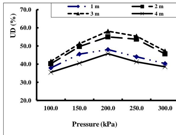
**Figure 2. Effect of pressure and UD for overhead floppy sprinkler.**
