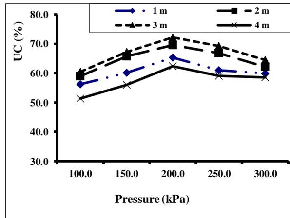
**Figure 1. Effect of pressure and UC for overhead floppy sprinkler.**
