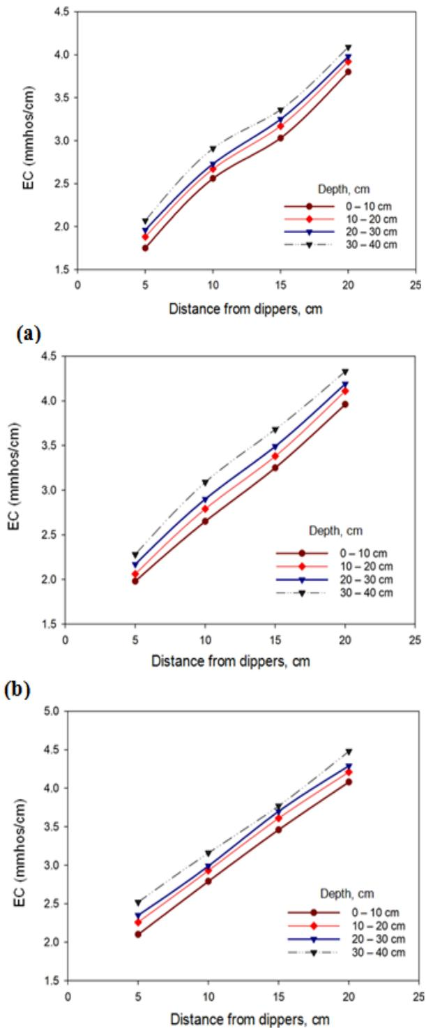
Fig. 3. Electrical conductivity distribution under drip irrigation system, at (a) 100, (b) 75, and (c) 50 %, soil salinity of total applied water
