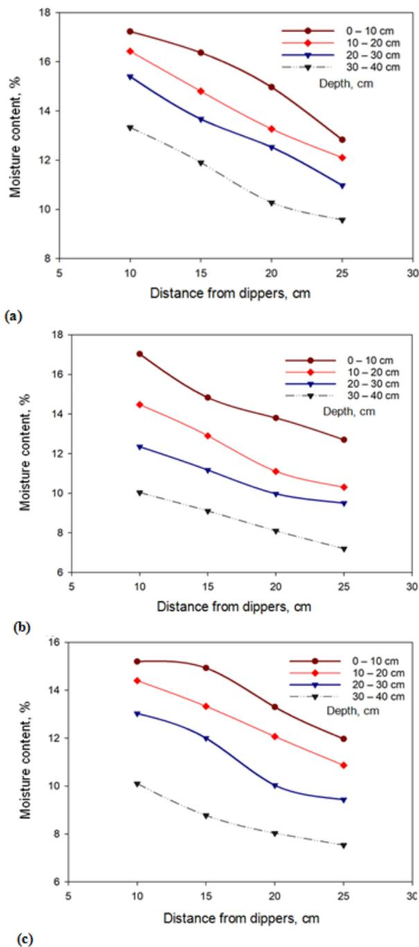
Fig. 2. Water distribution under furrow irrigation system, at (a) 100, (b) 75, and (c) 50 %, soil moisture of total applied water
