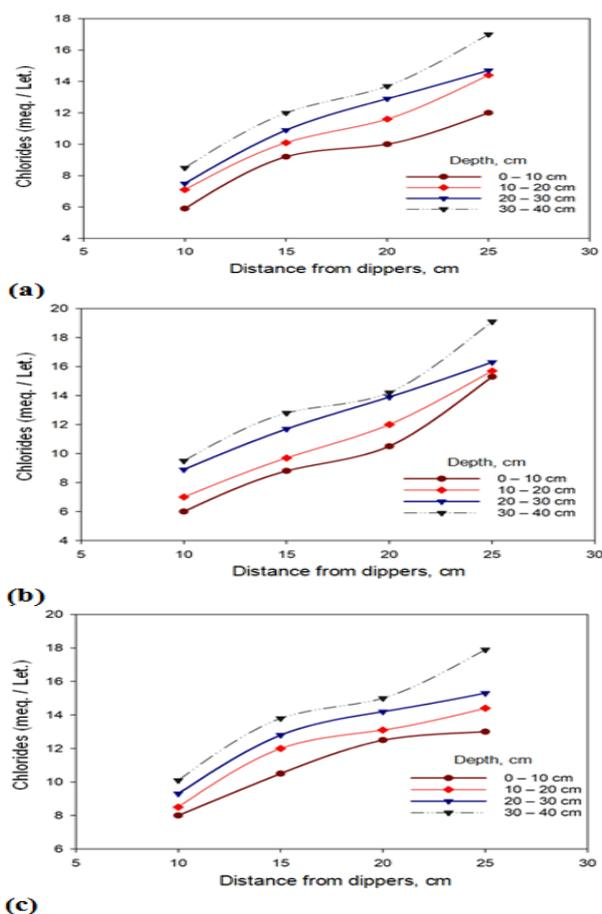
Fig. 6. Chlorides distribution under Furrow irrigation system, at (a) 100, (b) 75, and (c) 50 %, soil chloride of total applied water
