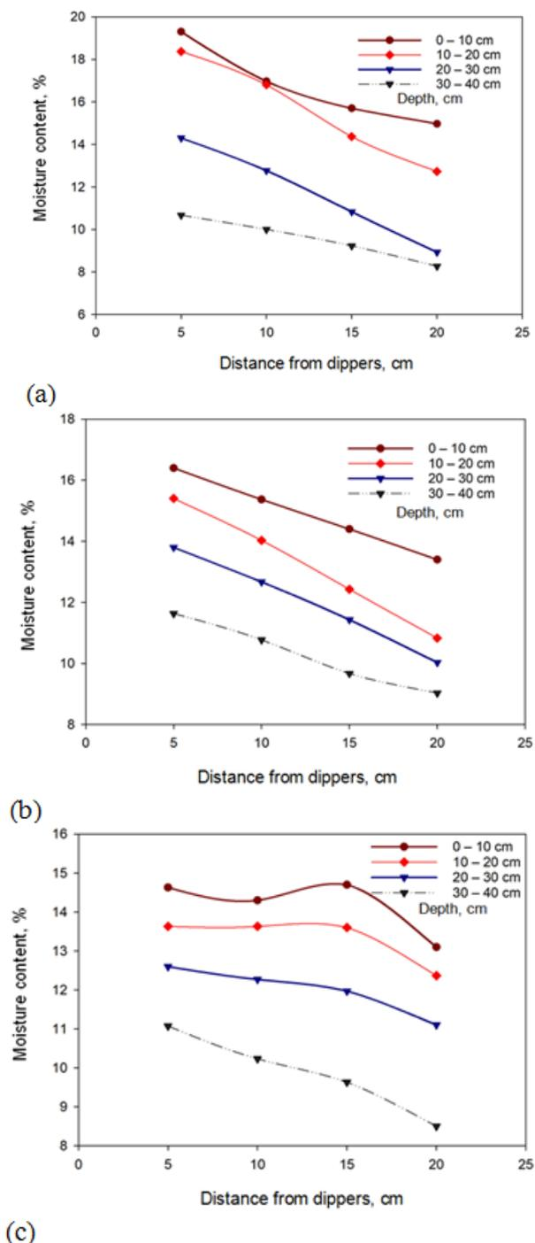
**Fig. 1. Water distribution under drip irrigation system, at (a) 100, (b) 75, and (c) 50 %, soil moisture of total applied water**
