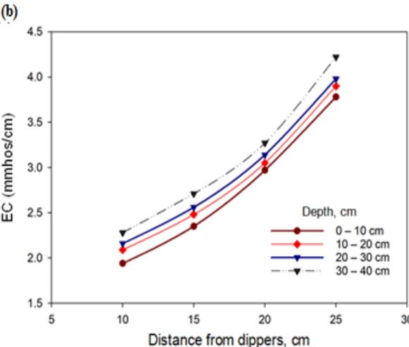
**Fig. 4. Electrical conductivity distribution under Furrow irrigation system, at (a) 100, (b) 75, and (c) 50 %, soil salinity of total applied water**
