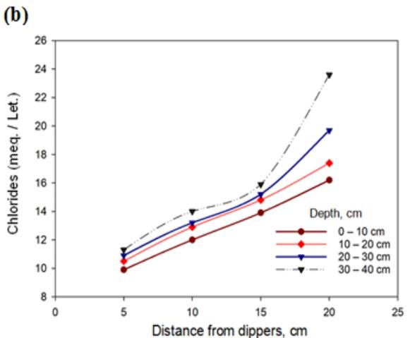
**Fig.5. Chlorides distribution under drip irrigation system, at (a) 100, (b) 75, and (c) 50 %, soil chloride of total applied water**
