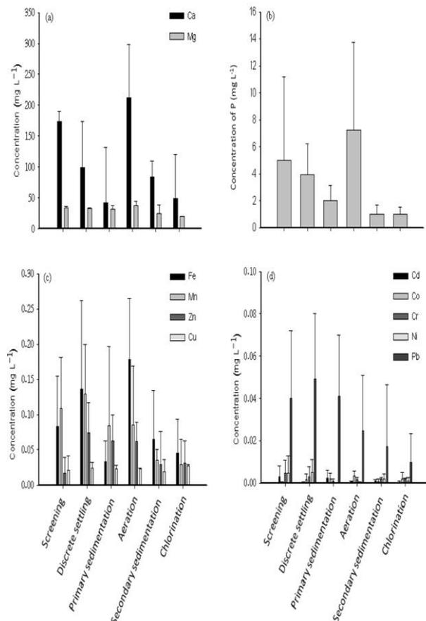
**Fig. 5. Efficacy of different processes used at wastewater treatment plants for the removal of Ca & Mg (a), P (b), micro elements (c) and heavy metals (d).**
