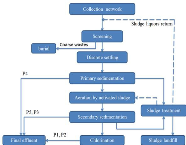
Figure 2. Schematic diagram of wastewater treatment processes used in studied units.
