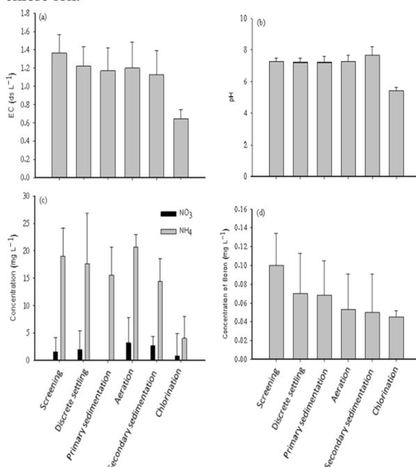
**Fig. 4. Efficacy of different processes used at wastewater treatment plants for the removal of salinity (a), acidity (b),  $\text{NO}_3$  &  $\text{NH}_4$  (c) and B (d).**
