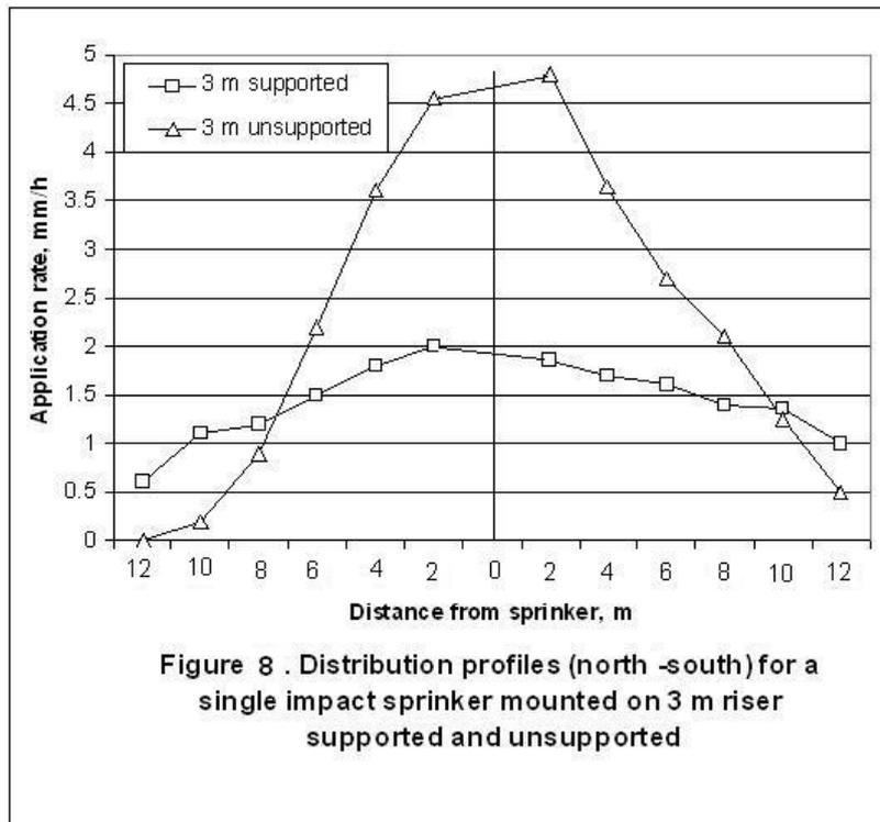
Which allowing sprinkler vibration, inclined from the vertical, thereby effectively increasing the trajectory angle. It may be concluded that well-supported risers made from steel pipe lead to very little vibration. Plastic pipe could be used as riser material, but it is more flexible and will undergo more vibration. To minimize riser vibration interference with sprinkler operation, plastic risers need to be rigidly supported.
