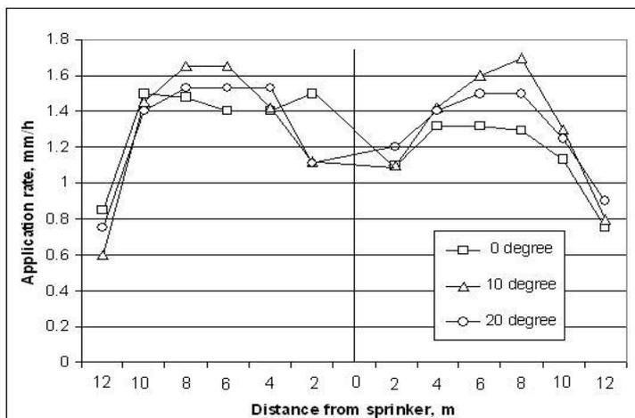
**Figure 5. Distribution profiles (west-east) for a single gear sprinkler placed at three different riser tilts**
