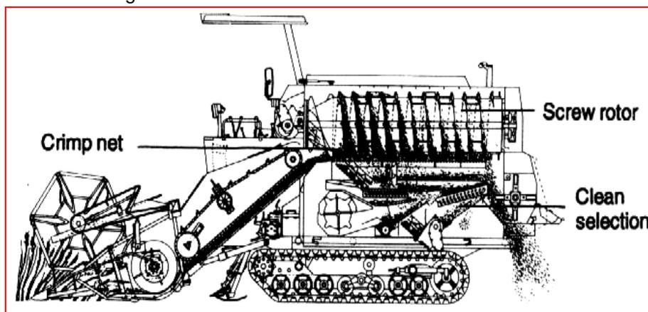
**Fig. 1: Cross section view of combine harvester (Yanmar-CA760).**
