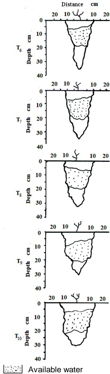
Fig (3): Soil moisture distribution with 100% of CWR
