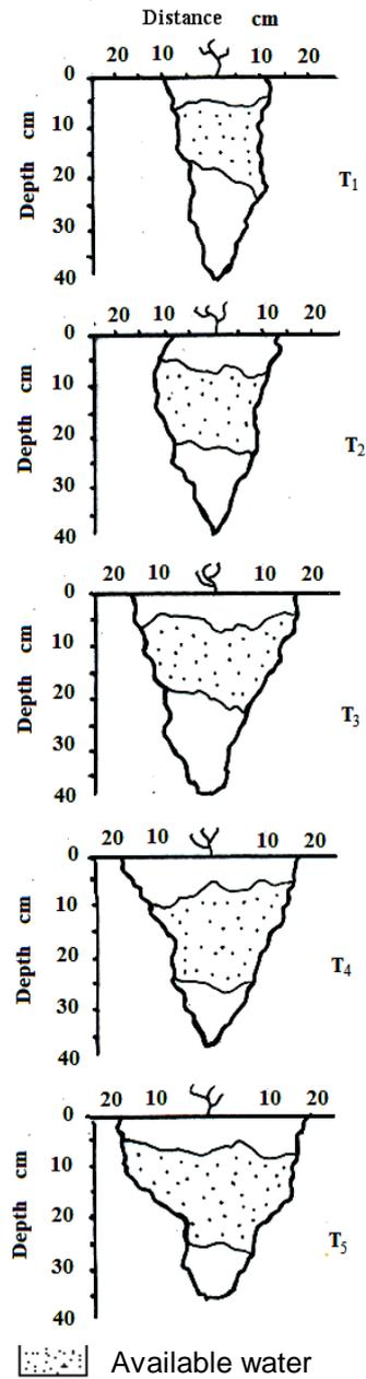
Fig (2): Soil moisture distribution with 80% of CWR
