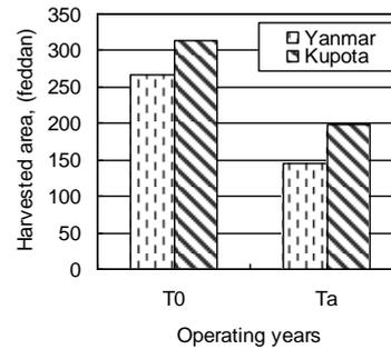
**Fig. (2): The average harvested area of two combines through and after the recommended salvage life ( $T_0$  and  $T_a$ ).**
