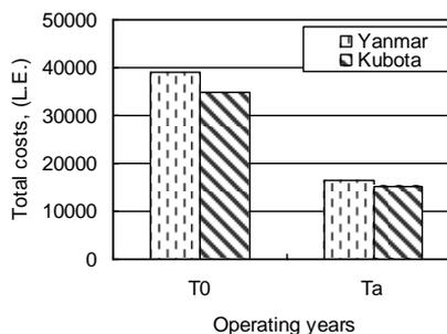
**Fig. (10): The average total costs of two combines through and after the recommended salvage life (T<sub>0</sub> and T<sub>a</sub>).**
