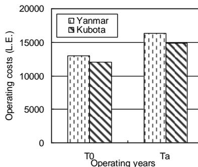
**Fig. (8): The average operating costs of two combines through and after the recommended salvage life (T<sub>0</sub> and T<sub>a</sub>).**
