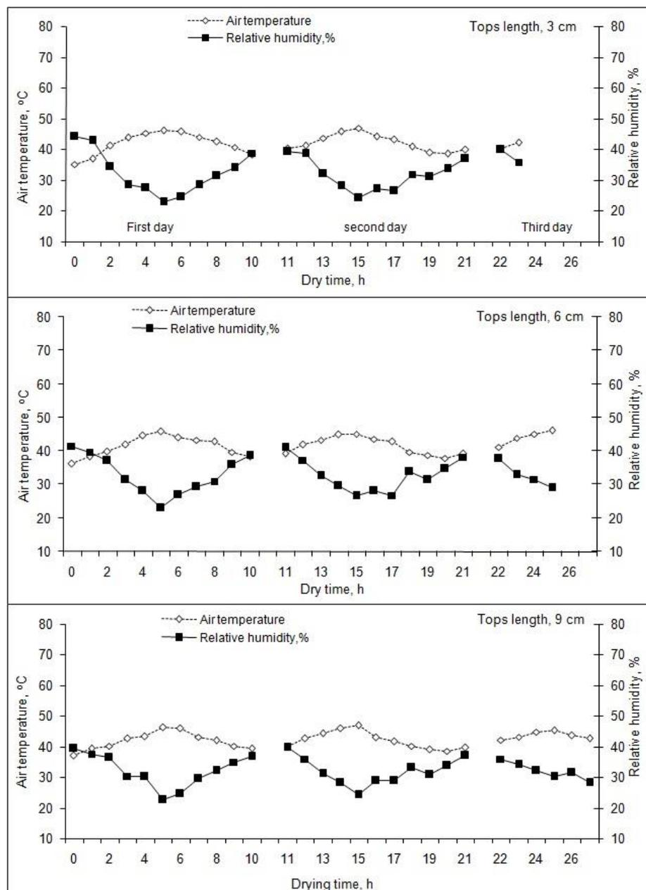
**Fig. (7): Air temperature and relative humidity as related to drying time using the maximum air velocity of 1.2 m/sec (chopped green tops).**
