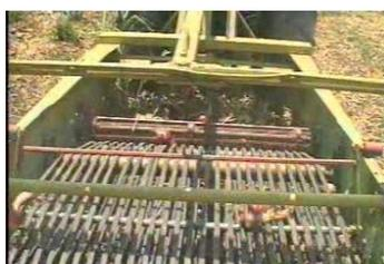
**Fig (6): The vibrator after development**
