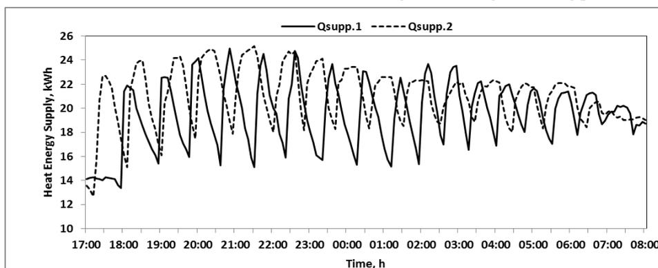
**Fig. 6. Cyclic changes in heat energy supply: (—) G1 and (...) G2.**
