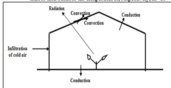
**Fig. 3. Schematic diagram of heat losses from the greenhouse**
