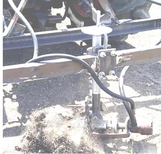
Figure 1. the spiral share with rotary axis
