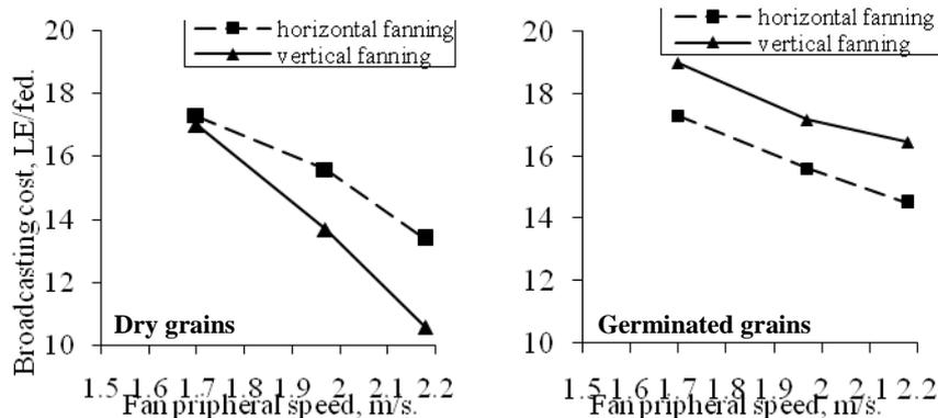
**Fig.7: Effect of fan peripheral speed and outlet pathlength on broadcasting cost under 200 mm outlet path length with dry and germinated grains**
