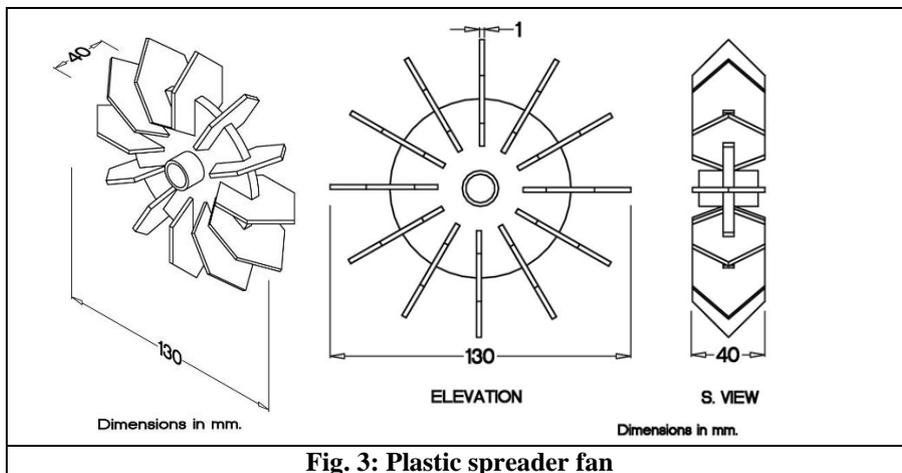
**Fig. 3: Plastic spreader fan**
