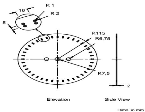
**Fig. 1: Schematic diagram of the vertical grain plate.**
