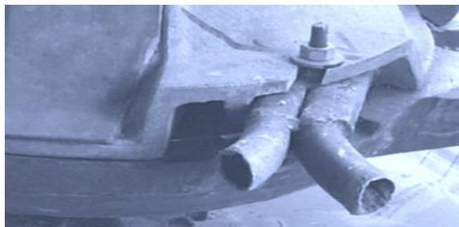
**Fig. 4: Photo of the grain delivery device**
