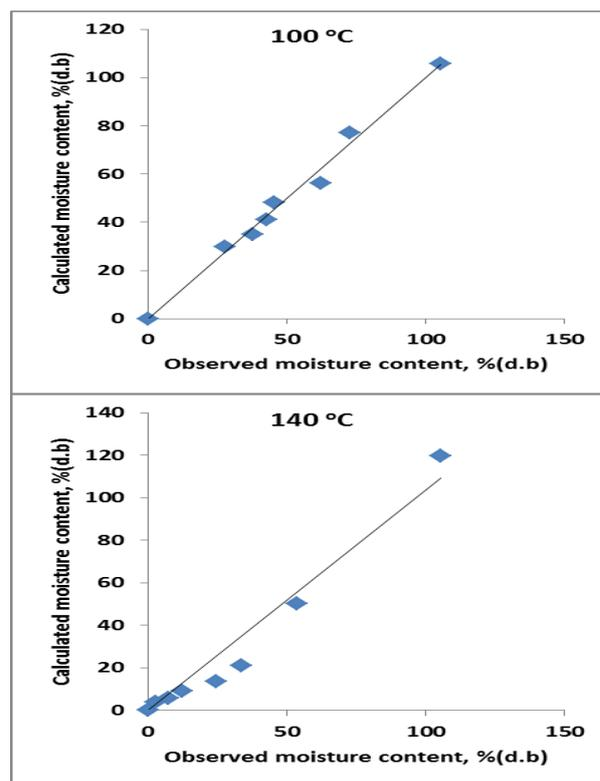
Fig. 6. The calculated and observed moisture content of orange pomace at heating surface temperature of 100 and 140°C for Henderson and Pabis model.
