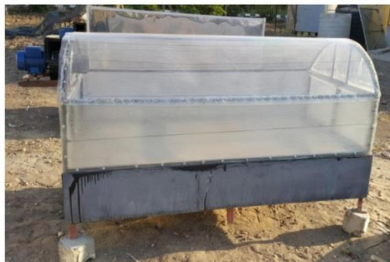
Fig. 1b. Modified-Quonset solar dryer
