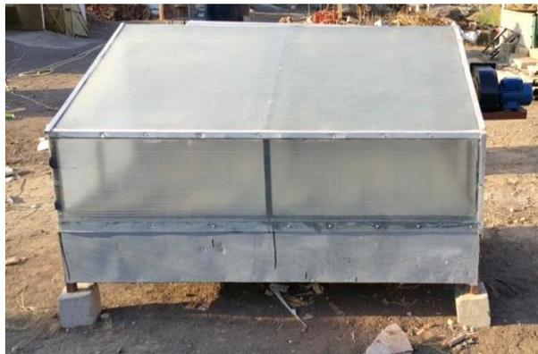
**Fig. 2b. Lean-to greenhouse solar dryer.**
