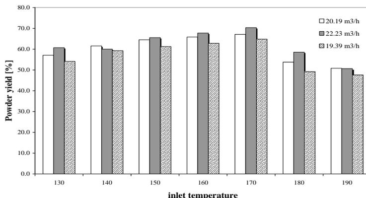
**Fig. 2. Powder yield [%] as a function of inlet air temperature and drying air flow rate for compressed air flow rate of 800 L/h.**
