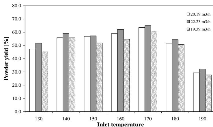
**Fig. 1. Powder yield [%] as a function of inlet air temperature and drying air flow rate for compressed air flow rate of 600 L/h.**
