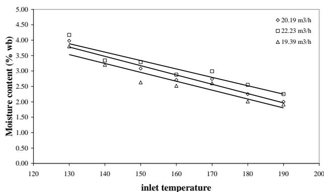
**Fig. 4. Powder moisture content as a function of inlet air temperature and drying air flow rate for compressed air flow rate of 800 L/h**
