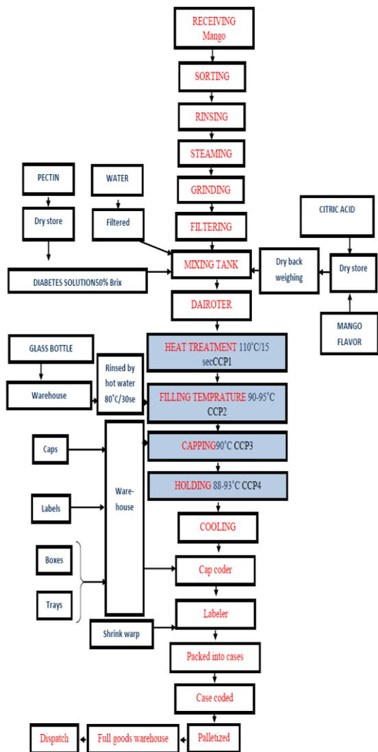
Fig. (2): Flow diagram of mango juice preparation.
