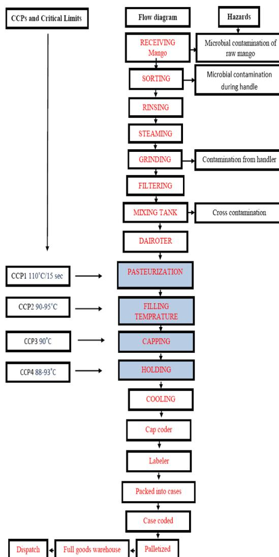
Fig. (3): HACCP Flow diagram of mango juice preparation.
