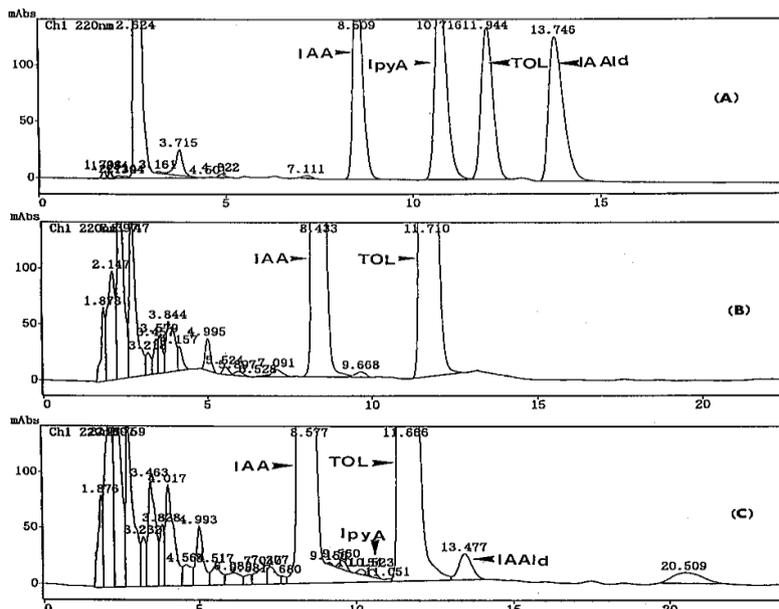
Figure 5: HPLC analysis of different auxins standard (A) and supernatants of 48 h. old cultures of *Azospirillum brasilense* Ft grown in N-deficient malate culture medium (B) and optimized yeast waste medium (C). IAA, indoleacetic acid; TOL, tryptophol; IAAld, indoleacetaldehyde and IpyA, indolepyruvate.
