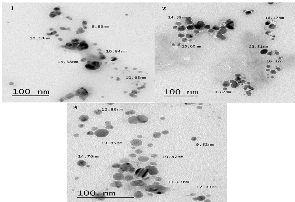
**Fig. 2. SEM image of spherical synthesized AgNPs by supernatants of growing *F. oxysporum* on different culture media: 1. potato dextrose broth medium, 2. Sabouroud broth medium and 3. malt yeast broth medium.**
