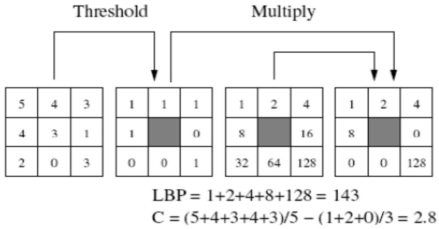
Figure 4. Computing the LBP and Contrast from [17]
