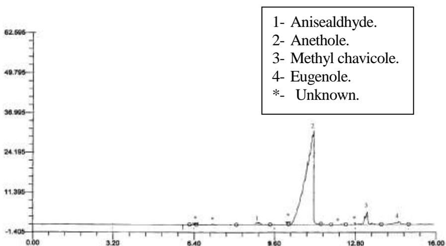
Figure 7. GLC chromatogram of anise oil (Phosphorene + Mycorrhiza + NPK 3).
