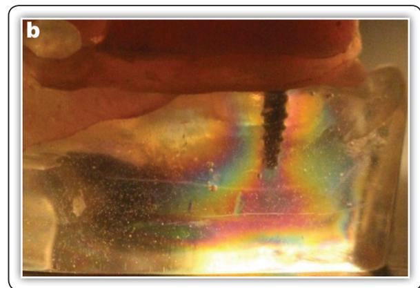
FIG (1) (a&b): Fringes order around dental implant with nylon framework under stress
