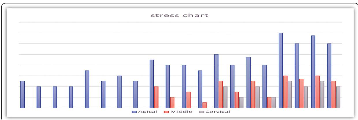
FIG (2): The stresses (20, 40, 60, 80, and 100 N) at apical, middle and cervical areas of left and right sides for two types of removable overdenture framework materials (nylon/metal).
