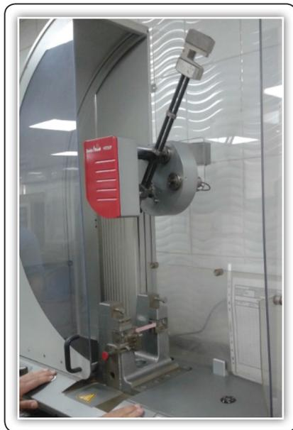
Fig. (1) Impact strength test.
