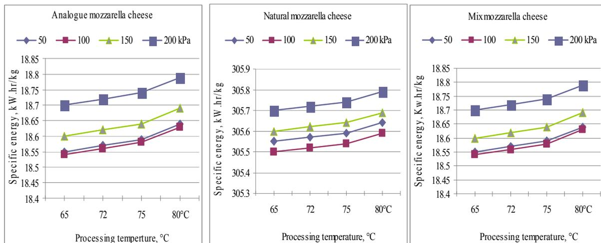
**Fig.7. Effect of processing temperature on the specific energy for producing analogue, natural and mix mozzarella cheese**
