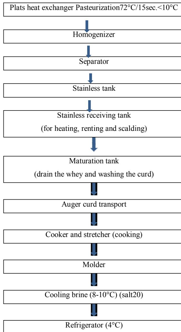
**Fig. 2: Flow chart of equipments used in natural mozzarella cheese production**
