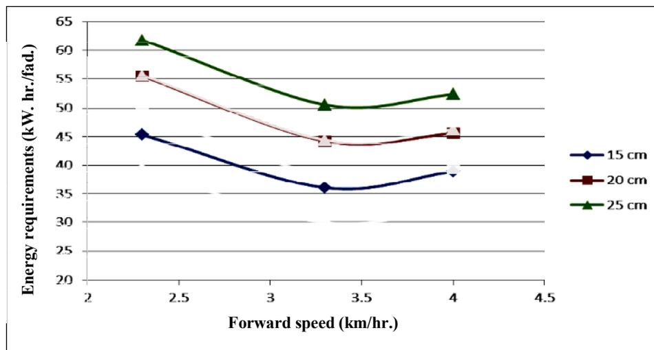
Fig. 13. Effect of forward speed and furrow depth on Energy requirements
