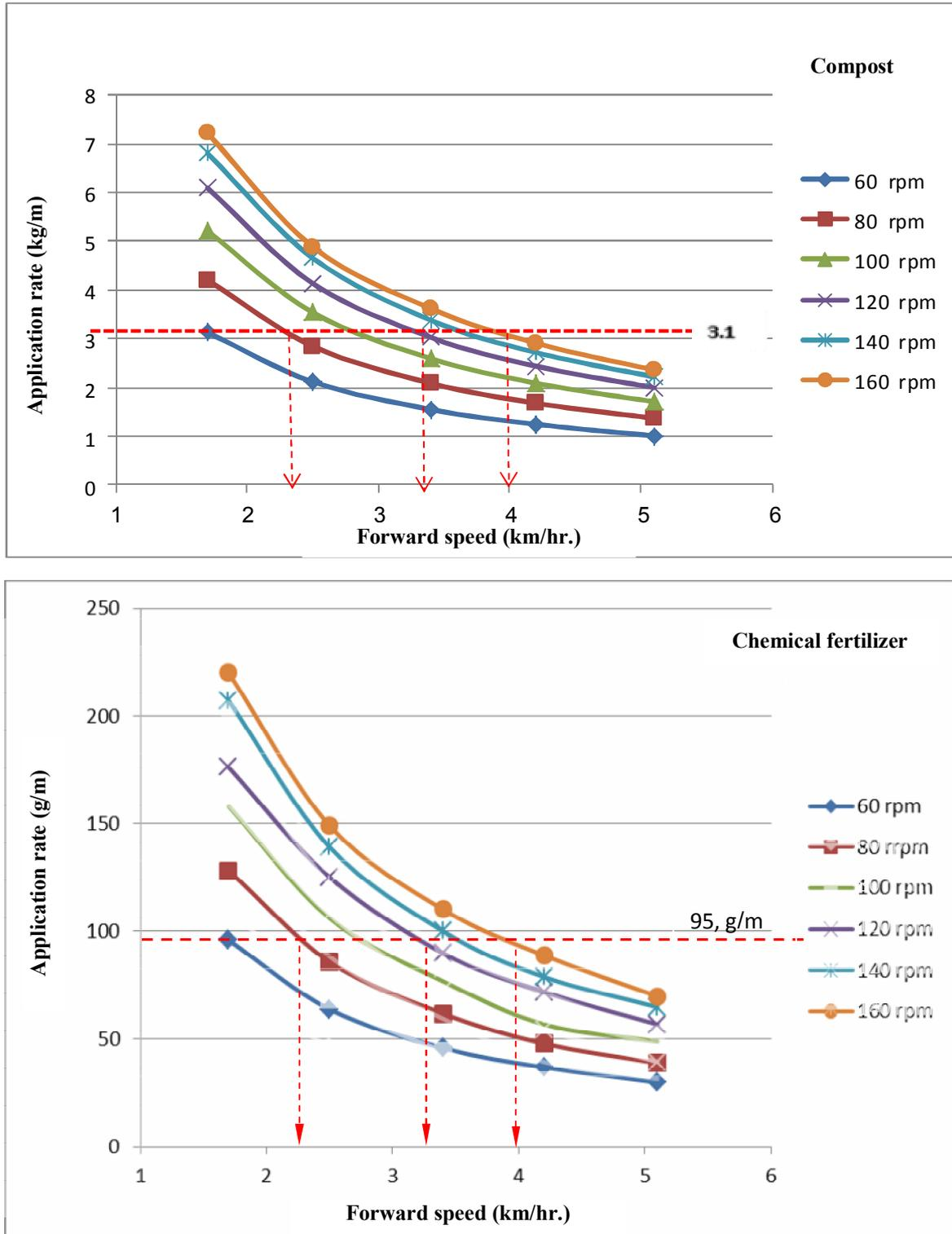
Fig. 5. Effect of feed shaft rotating speed and forward speed on chemical fertilizers application rate
