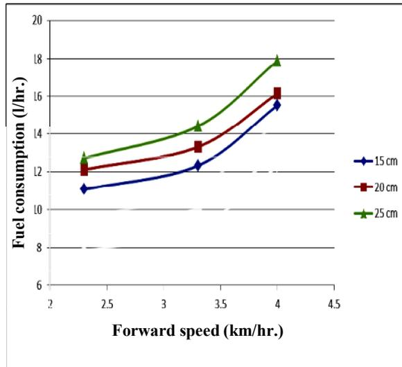
Fig. 11. Effect of forward speed and furrow depth on fuel consumption
