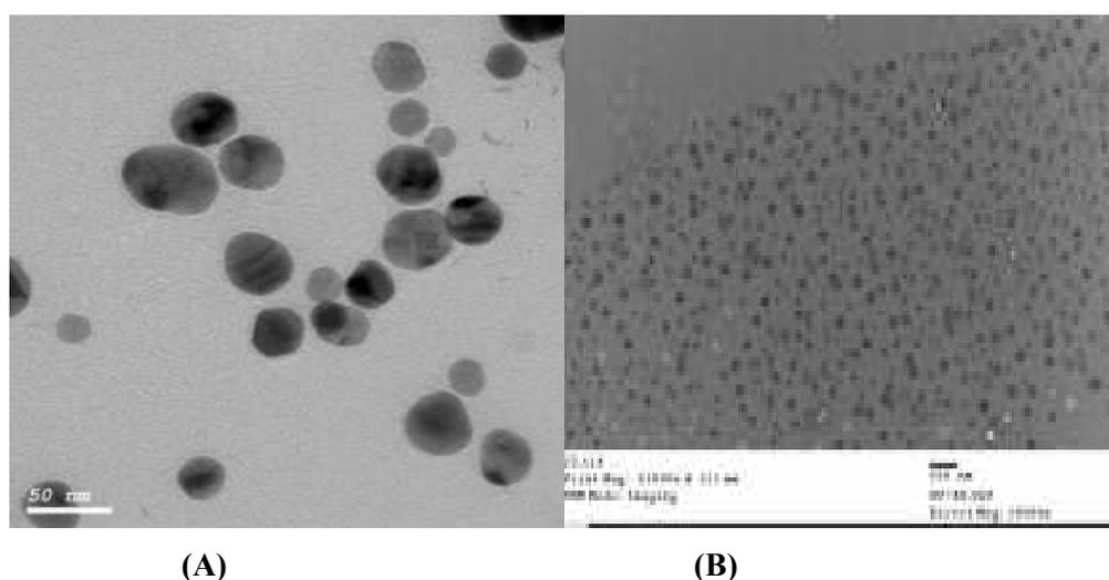
**Fig. 2.A. TEM micrograph of chemically synthesized silver nanoparticles, B. TEM image of chitosan nanoparticles**
