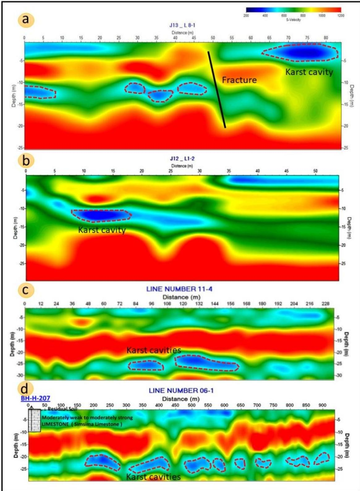
Fig.7. Selected study profiles show karstification within weak subsurface layers inside the study sectors and distribution of karst cavities within the area
