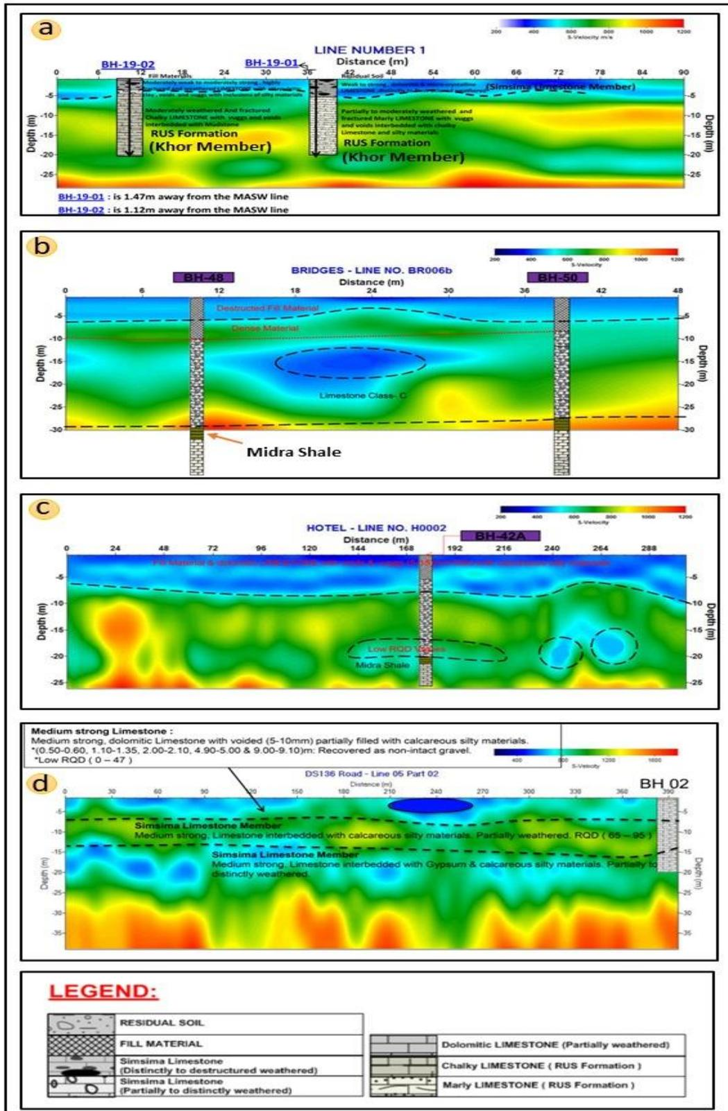
**Fig.6.** Subsurface profiles and correlation with the geotechnical boreholes to detect the subsurface layers and karst cavities within the layers
