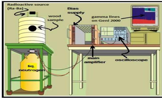
**Fig. 1:** Arrangements of HPGe Spectrometer System.
